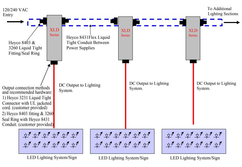
**Note:** All installations must conform toUL, Local and National Electrical Codes For NEMA 3 protection in outdoor installations, the use of Heyco liquid tight conduit and fittings (or equivalent) is required.
